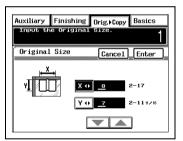
10 In the Original Size screen, touch X • , Y • , , and to specify the desired size, and then touch [Enter].
