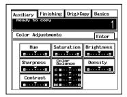
6 Touch the arrows to select the desired setting, and then touch [Enter]. (Ex: Hue adjustment)
