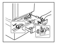
For "12-1/4 x 18" paper, adjust the trailing-edge guides as shown in the illustration.
