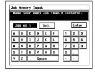
6 Check that the name for the selected job is typed correctly, and then touch [Exit].
